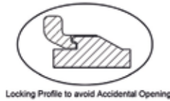
Locking Profile to avoid Accidental Opening
