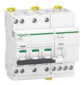
Residual current breaker with overcurrent protection (RCBO), Acti9 iCV40N, 3P+N, 10A, C curve, 6000A, A type, 30mA
