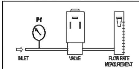
REFERENCE CURVE WITH AIR - Inlet pressure **P1 = 6.5 bar**
