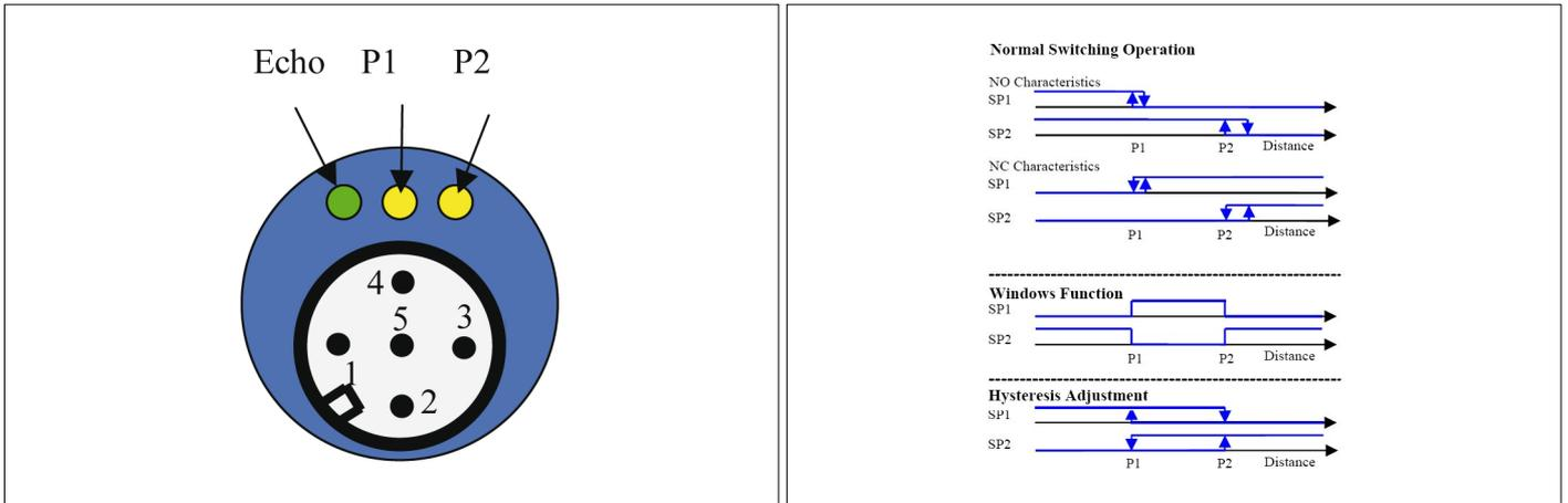
**3 different modes of switching outputs can be selected with this sensor:**
