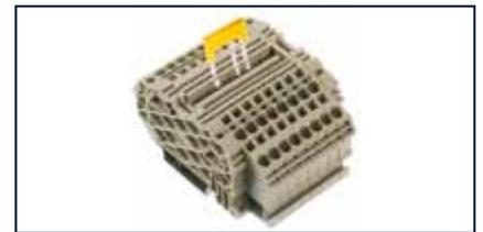
The cross-connection can be shorted using a cutting tool, but you must then make sure that the cut side is fitted with an end plate so that the voltage rating is maintained. For standard terminal blocks in the cross-section range from 2.5 mm<sup>2</sup> to 4 mm<sup>2</sup>, it is adequate to attach the **ZQIs** in an offset position (with two cross-connection channels).
