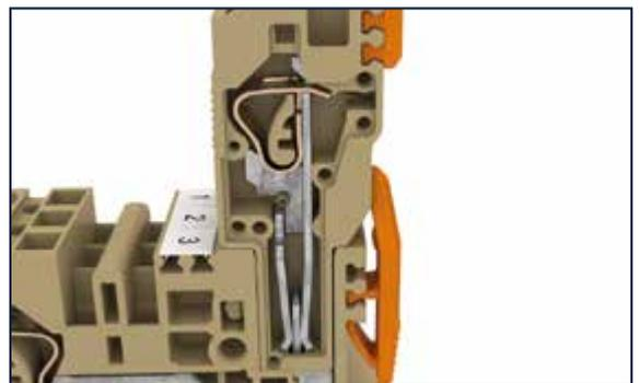
The base terminals and the pluggable versions are designed so that they are finger-touch safe. This feature provides excellent protection for the user and also permits power to be fed-in via the terminal or the plug.
