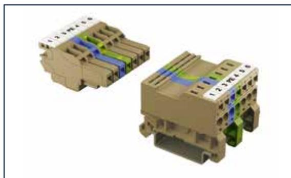
Effective wall bushings can be constructed simply by snapping the **ZST-WA** wall-bushing mounting adapter onto the **ZSTK 2.5/.../B** coupling element. These multi-pole units snap on sideways to the wall; the pressure on the inner slide mechanism ensures a secure attachment to the housing! The outer connector unit can be optionally fitted with locking elements.
