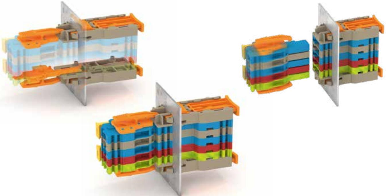
Effective panel feed-through bushings can be constructed simply by snapping the **ZST-WA** mounting adapter onto the **ZSTK 2.5/.../B** coupling element. These multi-pole units snap on sideways to the wall; the pressure on the inner slide mechanism ensures a secure attachment to the housing. The outer plug unit can be optionally fitted with locking elements.
