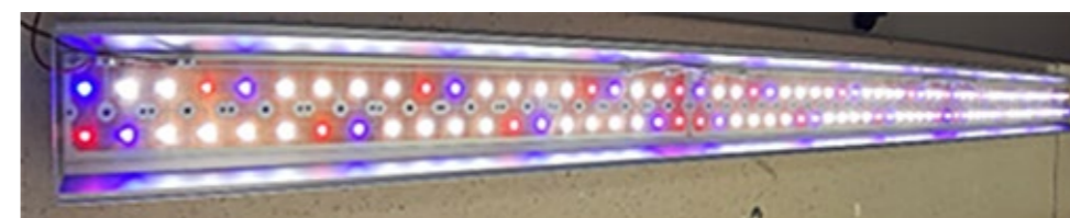
Pic. 6. Horti A luminaire for seedlings.
