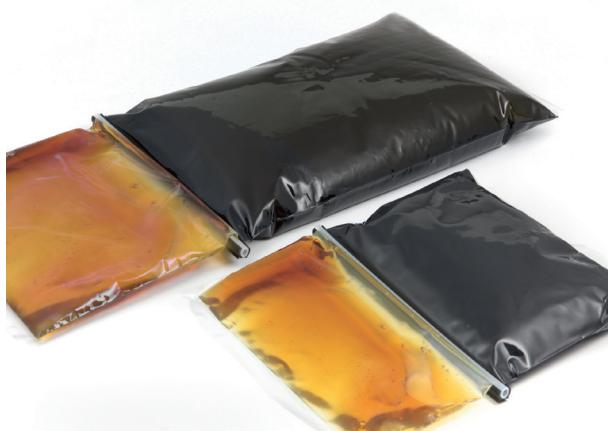
Filofill PC5581 is specially designed for cable joints up to 3.3kV. PC5581 has good anti corrosion properties and shows a good adhesion to metals, ceramics, and many different plastics, and can be utilized on all plastic- and paper insulated cable types.
