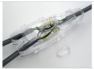
The Filoform range of cast resin Branch Joints are approved in accordance with DIN EN 50393 (VDE 0278:393):2006-11, and are suitable for use with both armoured and unarmoured cables up to and including 1kv. The joints are suitable for use on most cable types, including PILC, XLPE, PVC and EPR, and can be supplied complete with armour earth kit and mechanical connectors as standard.
