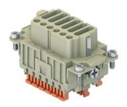
Female insert, CDSH series, SQUICH® spring terminal connection without tools, 18 poles + PE, 10 A 400 V 6 kV 3, size "57.27"
