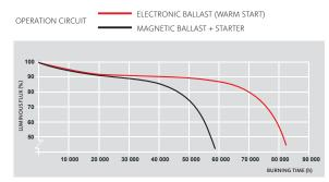
Service Life is reached when the amount of light in an installation falls to 80% of the initial 100 h value. The Service Life of the lamp failure rate and the lumen depreciation is calculated according to IEC/EN 60081 which is based on a 3 hour operating switching cycle.
