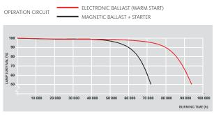
The lifetime with a 12 h switching cycle is defined as; the time when 10% of the lamps in an installation have failed. The lumen depreciation at this time is indicated with less than 10%.
