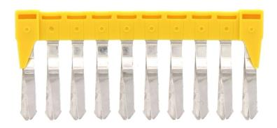
Insulated cross-connector, No. of poles: 10, Mounting type: Plug in, Width: 50.7 mm, Rated cross-section: 2.5 mm², Colour: Yellow
