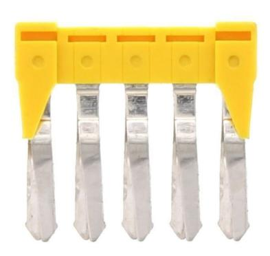
Insulated cross-connector, No. of poles: 5, Mounting type: Plug in, Width: 25.2 mm, Rated cross-section: 2.5 mm², Colour: Yellow
