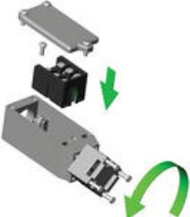
Designed with a removable lid to fit replaceable contact blocks. For extra durability flexible actuators are available.
