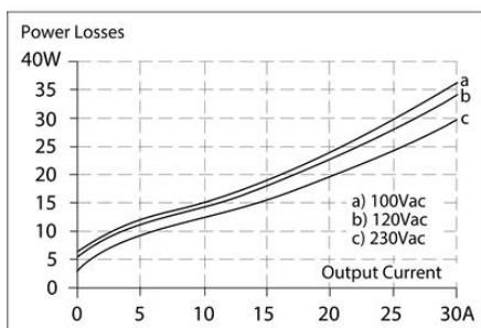
Fig. 9-2 Losses vs. output current at 12V, typ.
